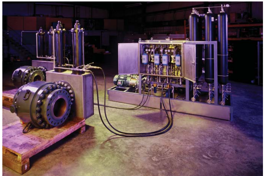
HPA-3002.HV Lockhopper System for Coal Gasification Gasifier Vessel (3-second operation)
