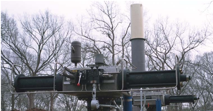
QT-40.280 High Pressure Gas Actuator with GE-5000 electrically piloted controls and hydraulic manual override
